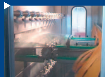
Glass in the final rinsing zone
