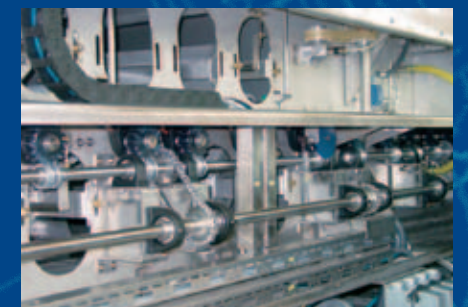
Maintenance-free stainless steel worm drive
