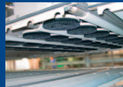
Two to four oscillating polishing gantries
